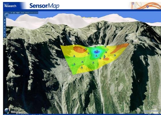
Fig. 4. Spatial visualization of ambient temperature measurements from the Le Genepi deployment. SensorMap generates this type of contour map on request and overlays it on top of 3D high resolution maps. Users clearly see the interaction between ambient temperature and the terrain.
