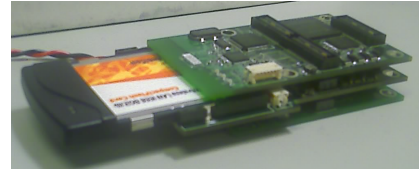
Figure 1. An mPlatform node with the 802.11 and 802.15.4 radios.
